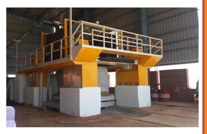
Rosava Engineering has gained huge recognition in offering high quality Gang Saw Machine that requires less maintenance and can be easily installed. It is used in the cutting and processing of Marbles & Granities. The offered machine is fabricated using premium quality components and advanced technology in compliance with the international quality standards. This machine is available in various technical specifications to meet the diverse needs of the clients.
